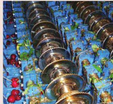
Above Major problem areas in the packing line: large fruit drops (top) and cluster cutters (above) responsible for pitting damage.
