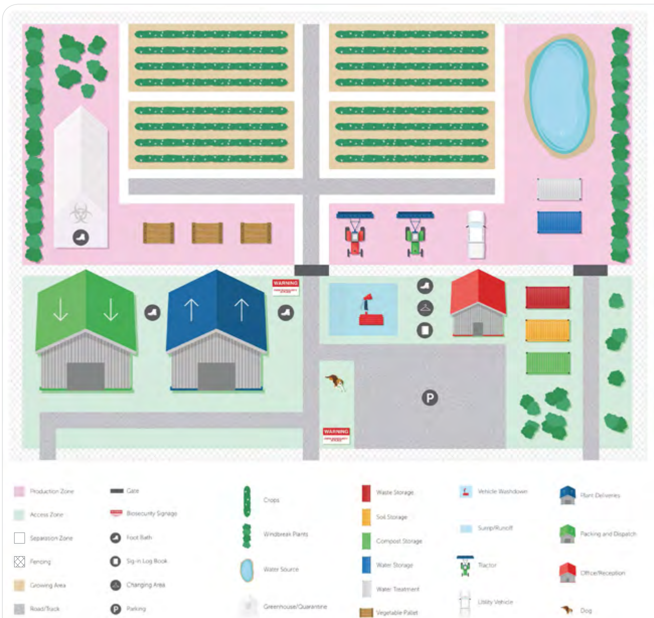
This map shows the relative positions of some facilities found on a farm in relation to the best place to put features like signs, parking or washdown areas. Green represents access zones, grey or white represents separation zones and pink represents the farming (production) zone.
