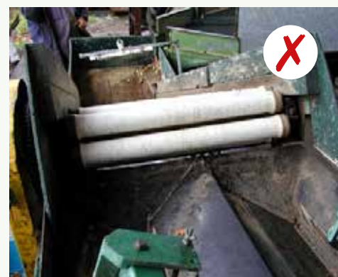
Figure 22 – Packing line equipment should be easy to clean: porous materials such as carpet must not be used, gaps that can accumulate debris should be avoided and packing lines must not have loose or flaking paint.
