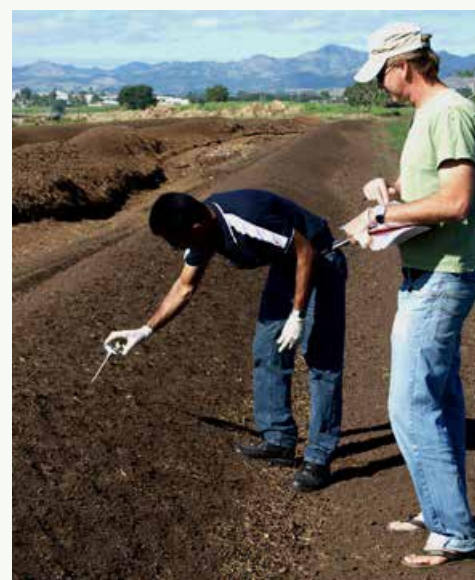
Figure 11 - Treating compost containing manure involves keeping the pile well aerated by turning at least three times, with a minimum of 3 consecutive days at \geq 55^{\circ}\text{C} between each turning event (Trac-turn, AusTech).
