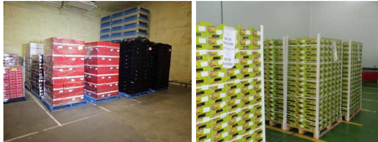
Figure 25. Use of fibreboard boxes with stretch wrap and returnable plastic crates (RPC) on pallets (left) and fibreboard boxes with pallet corners to increase pallet strength (right) in packinghouse coolroom awaiting distribution to market.
