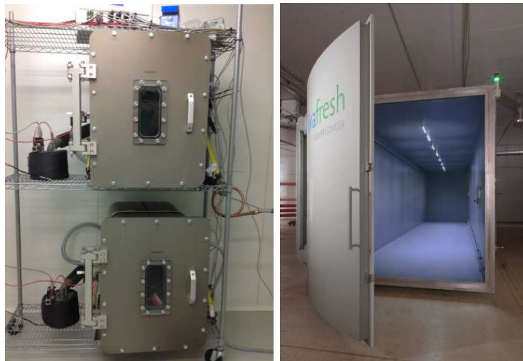
Figure 57. Experimental low pressure chambers for postharvest storage and disinfestation research at NSW DPI, Ourimbah (left). Commercial low pressure shipping container(right) – VivaFresh™ (USA).
