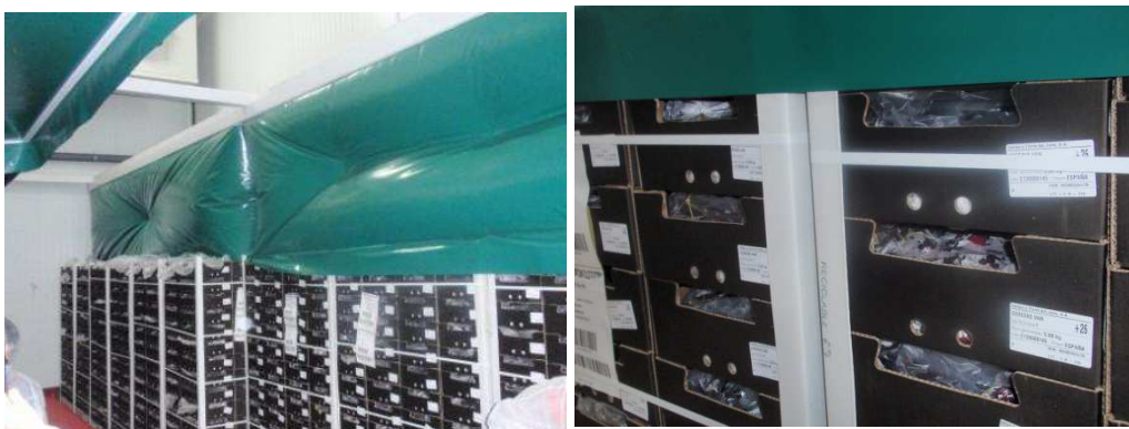
Figure 11. Post-pack cooling of cherries in packed sealed boxes for storage and marketing in Spain. Note forced air cooling of the fruit with some ventilation holes in the boxes to allow air flow / cooling. (Photos - John Golding, NSW Department of Primary Industries)
