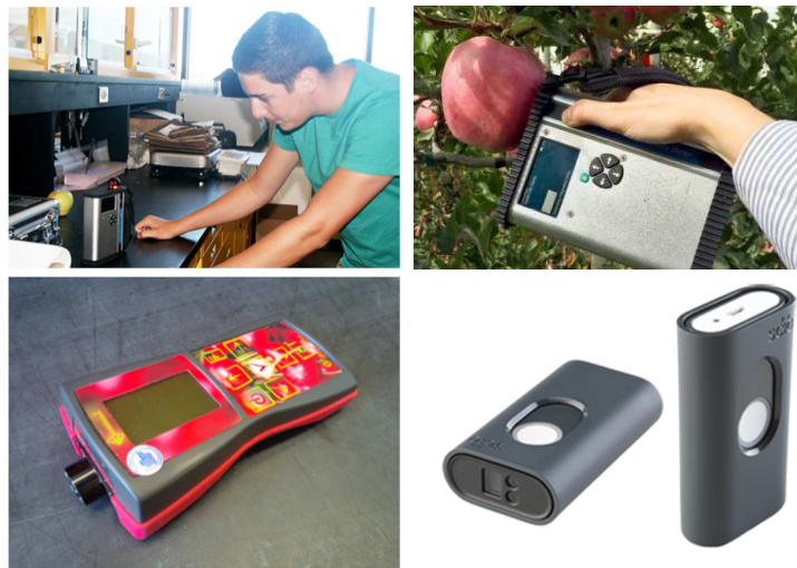
Figure 59. Use of Felix 750 hand held NIR instrument for laboratory testing of cherries (top left) and field / orchard (top right), DA cherry meter (bottom left) and SCIO pocket spectrometer (bottom right).
