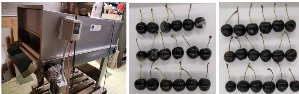
Figure 56. Prototype custom made semi-commercial in-line UV-C treatment at NSW DPI, Ourimbah (left). Results of treatment of 'Sweetheart' cherry fruit with UV-C light stored at 20 °C – untreated control (middle) and 50.8 kJm -2 UV-C treatment (right) (from Pristijono et al., 2018c). (Photos – Penta Pristijono University of Newcastle)
