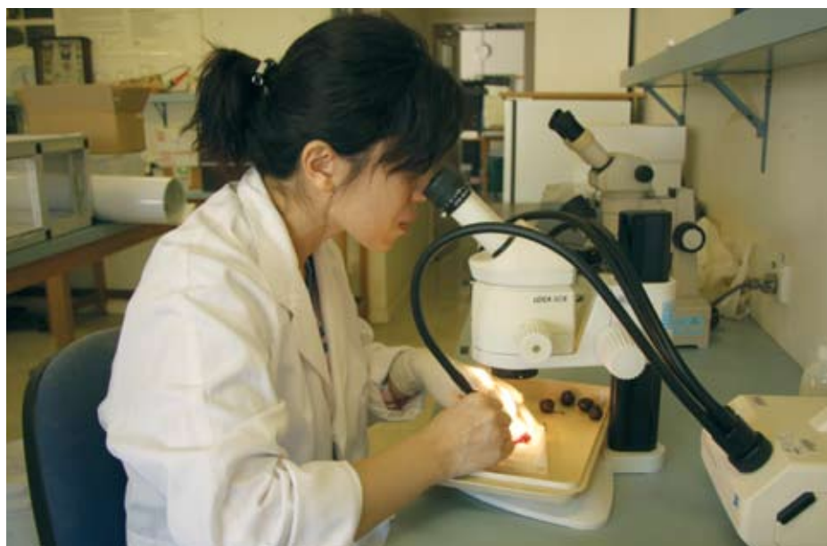
BAPHIQ Inspector examining cherry fruit for surviving QFF larvae following treatment at 3°C for 14 days.
