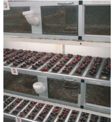
Infesting cherry fruit with Queensland Fruit Fly before disinfestation treatments and cold storage at I&I NSW
