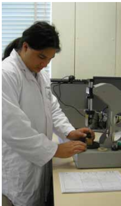
Honours student measuring firmness with the Guss fruit flesh texture analyser on fruit sampled for the nutrient matrix study
