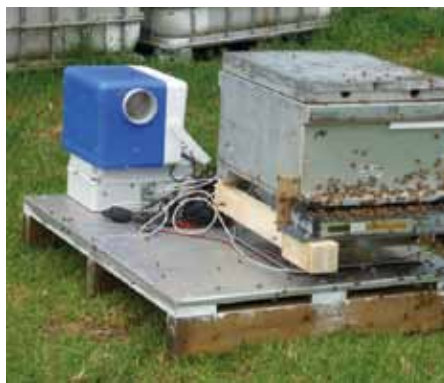
Monitoring the arrival of a swarm of bees to a bait box instrumented with cameras and weight, temperature and relative humidity sensors in controlled trials
